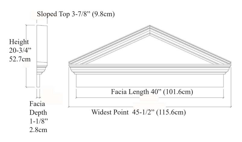
Made from Arch-Polymer<sub>TM</sub> Interior & Exterior, White Primed, High Quality, Cuts like Wood Similar density to White Pine
