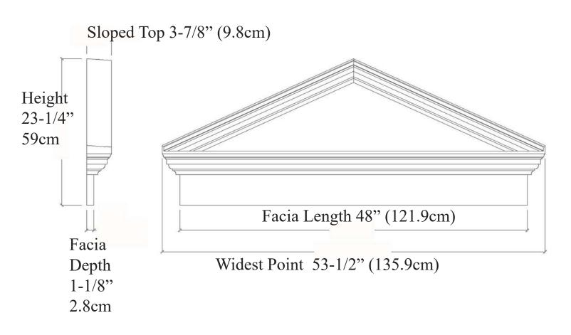
Made from Arch-Polymer<sub>TM</sub> Interior & Exterior, White Prime
