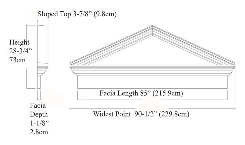
Made from Arch-Polymer<sub>TM</sub> Interior & Exterior, White Primed, High Quality, Cuts like Wood Similar density to White Pine, Rot, Water & Insect Resistant, Easy to Install
