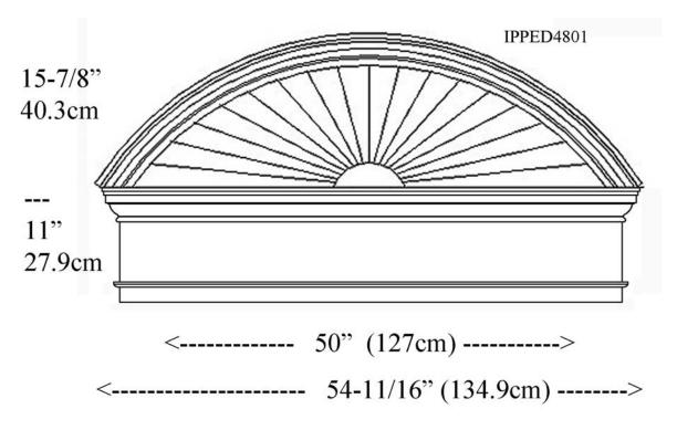
\* assembly required, drawing not to scale
