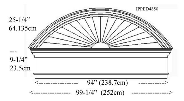
\* assembly required, drawing not to scale
