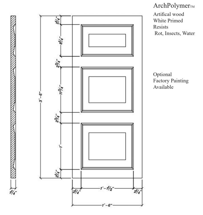
\* assembly required, drawing not to scale, mounting hardware by others
