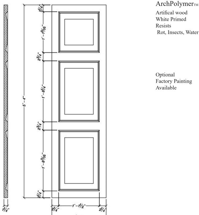
\* assembly required, drawing not to scale, mounting hardware by others
