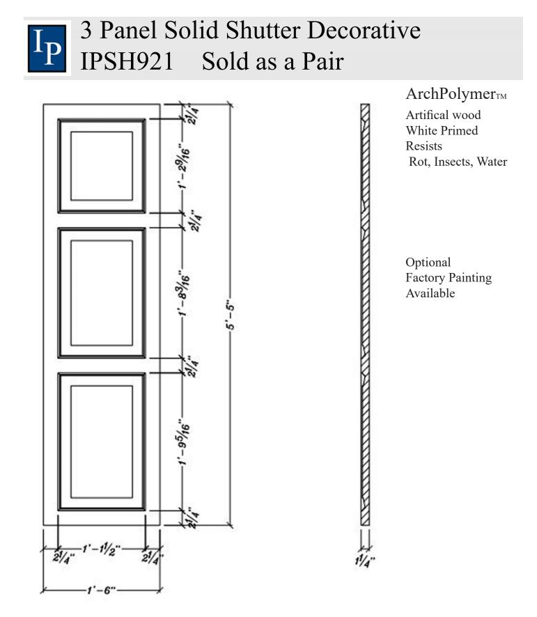
\* assembly required, drawing not to scale, mounting hardware by others
